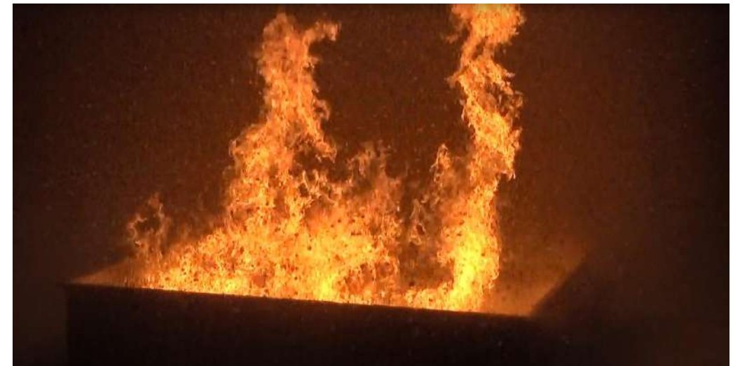
Fomtec Enviro USP applied through nozzle "B"
