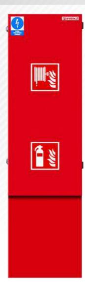
Hydrant cabinet insulated by material with thermal conductivity 0.0359 [W/m\*K] 150W heating element with thermostat, 230V
